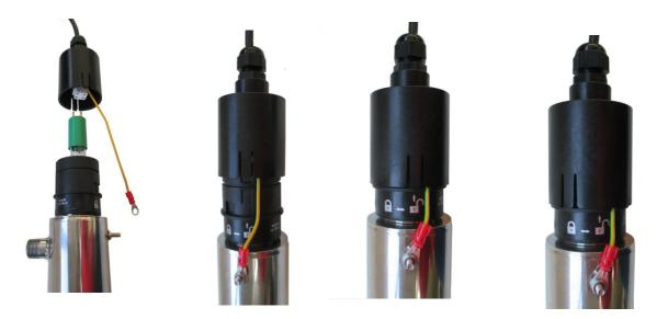
Finally connect the power cable to the socket.
